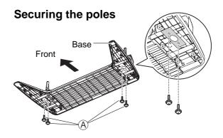
Use the assembly (A) screws to secure the poles firmly to the bottom of the base.
